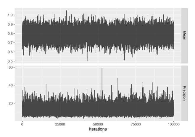
For both variables the trace should look like 'random noise', as is the case above. When we see auto-correlation, meaning that one value of the trace depends on the previous value of the trace, the MCMC might not be reliable and we should not trust the 95% credible interval.
