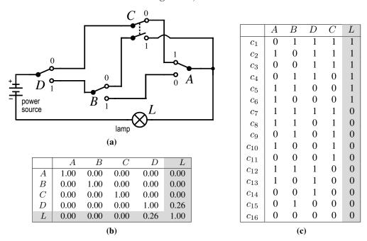
Figure/Table 2: Diagram (a) depicts a simple electrical circuit with three single-pole switches D, B, A, one double-pole switch C, and one lamp L. Table (c) comprises ideal data on that circuit and Table (b) the correlation matrix corresponding to that data.
