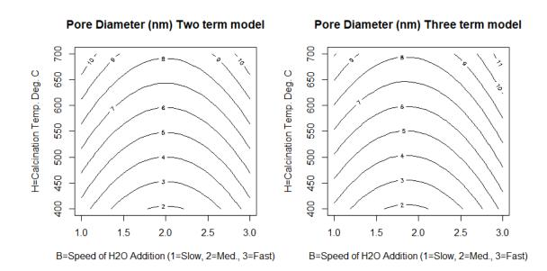
Figure 2: Contour plot of TiO2 Pore Diameter.
