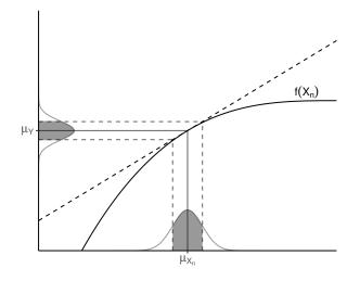
Figure 1: Illustration of linearity in an interval  $\pm$  one standard deviation around the mean.
