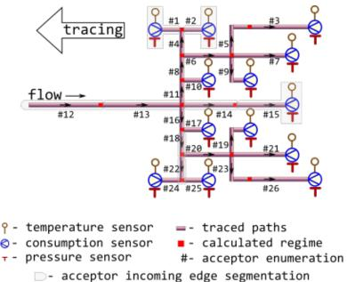
Tracing starts from sensor-equipped nodes and goes backwards, i.e against the flow direction.
