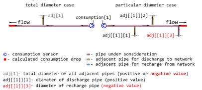
Usually, there are no additional sensors that could measure consumption in each flow fork. In that case they only may operate with geometric factors, i.e. assuming that flow rate is proportional to square of pipe diameter.
